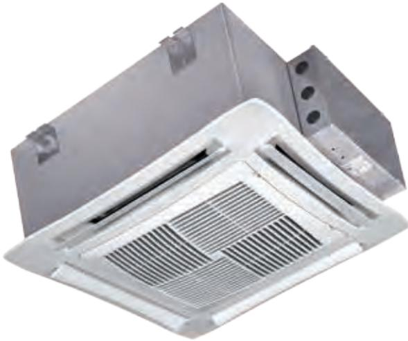
The **ELFOSpace BOX2** terminal unit has been designed for installation in suspended ceilings without requiring any extra part for operation. The unit has an intake grille and four-way outlet with adjustable diffuser flaps for changing airflow direction.
